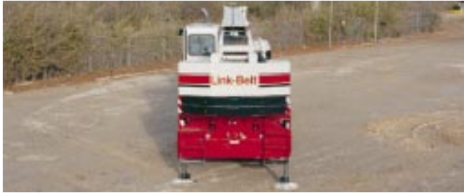
Retracted Outriggers 7' 9" (2.36 m) Spread
