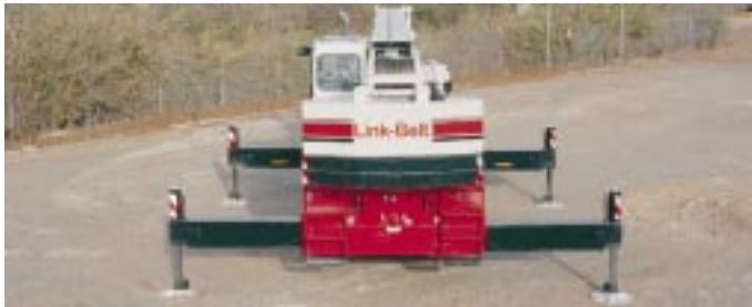
Fully Extended Outriggers 20' 6" (6.25 m) Spread
