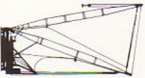
Heavy Lift Crawler Cranes 360 tons
