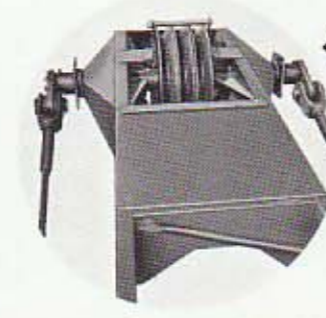
THREE SHEAVE HEAD MACHINERY for either standard angle boom or optional "HI-LITE" boom features three boom-point sheaves mounted on anti-friction bearings. No need to lower boom for daily greasing. Triple sheaves permit multiple reeving of hoist line for extra fine control in spotting loads. Jib peak sheaves also on anti-friction bearings.
