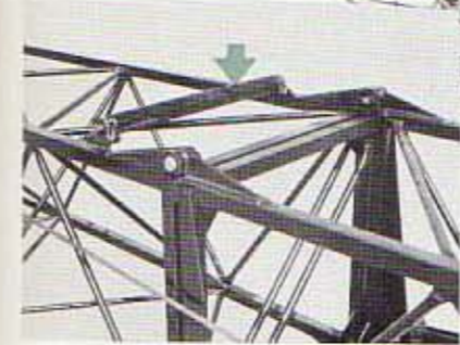
CABLE SUPPORTING ROLLERS are required when a third drum cable passes over crane boom. One roller is furnished as standard for "Hi-Lite" booms, 40 feet to 100 feet long. These rollers, full width of boom and mounted on anti-friction bearings, protect any long boom from cable slap or wear, also give longer cable life.
