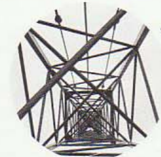
A STUDY IN SYMMETRY is this end view of the optional "HI-LITE" tubular boom. Pyramid-like, tetrahedral cross bracing design cuts long boom deflection and whipping action to a safe minimum. The four main chords are sealed square tubes of high-strength, light-weight alloy steel. Lattice-work and internal cross bracing are of sealed, round tubing.
