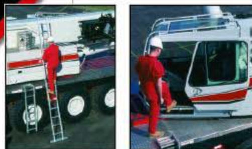
Access ladders with hand rails and a large flat deck are standard on Link-Belt cranes, providing superior accessibility.
