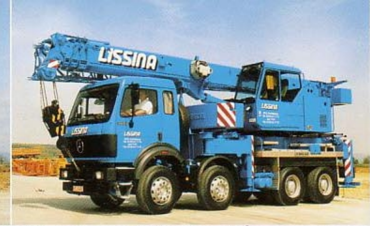
Telescopic crane LTF 1030-4 mounted on a 4-axle Daimler-Benz chassis type 3334 K / 8 x 4.
