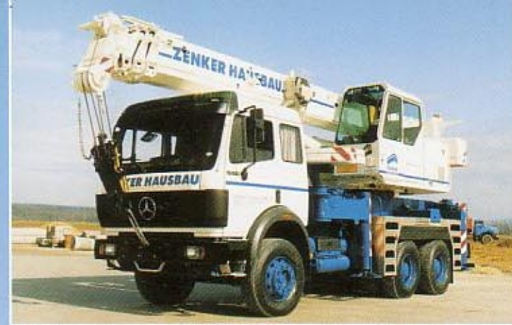
Telescopic crane LTF 1030-3 mounted on a 3-axle Daimler-Benz chassis type 2631 K / 6 x 4.
