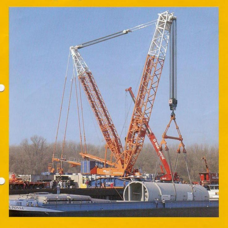
For the teams of crane operators Riga-Eisele, Mainz and Frankfurt as well as for the heavy-duty experts of Messrs. Baumann, Bornheim, it was a project of the superlatives: The transport of a reactor of 450 tons with a length of 32 meters from Mannheim to Neustadt on the river Danube as well as the subsequent positioning
