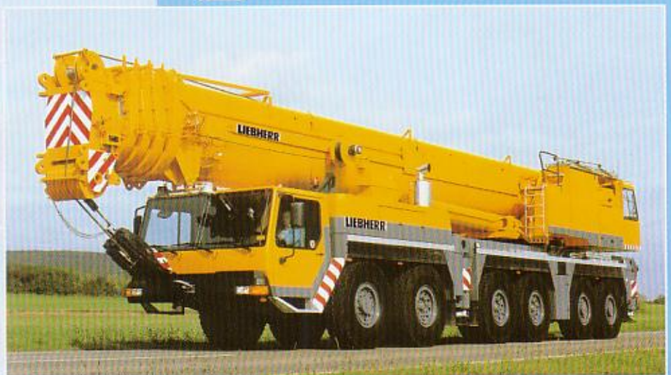
Mobile crane type LTM 1300/1
