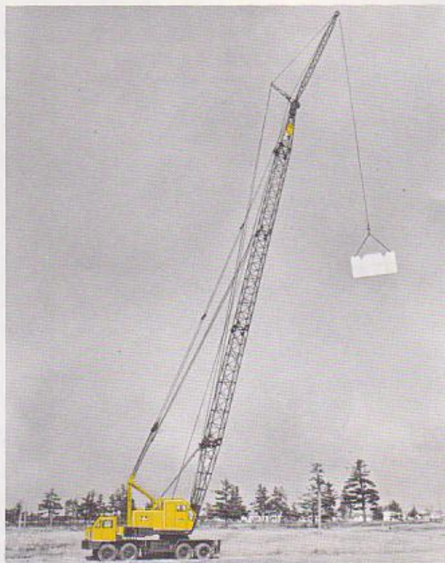
LONG REACH — The 440-TC easily handles up to 200 feet of T-1 steel boom and jib.
