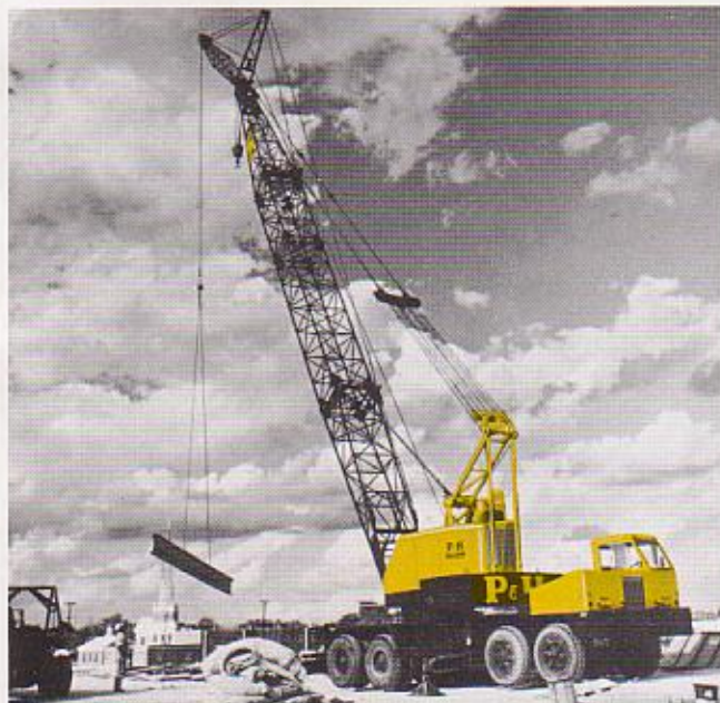
STABILITY — Hydraulic outriggers set up carrier fast into a stable, solid working platform.
