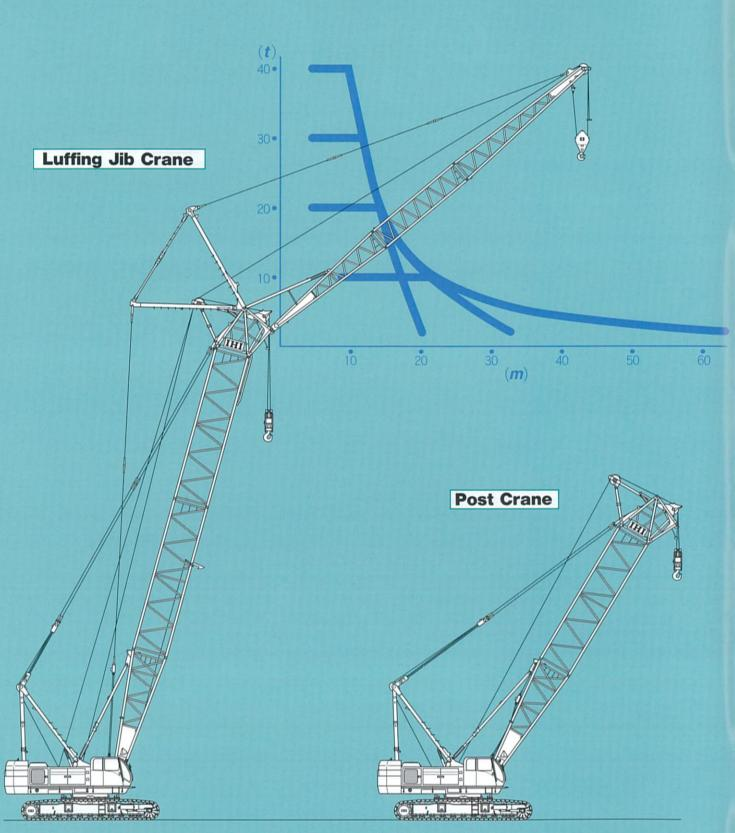
Main and Jib hook blocks may not be operated simultaneously.
