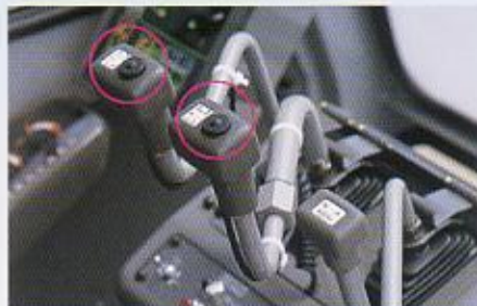
Fine Inching with the Lever-mounted Drum Rotation Sensing System
